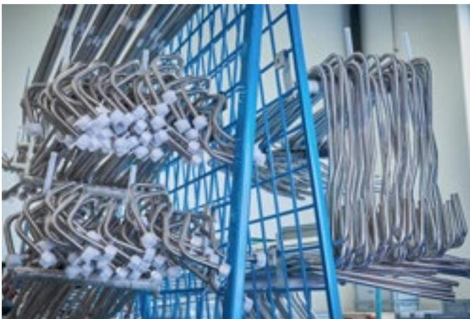
The tubes are bent and assembled in economical lot sizes. Delivery is made on time and in the agreed quantities directly to the customer, and can be incorporated in the production cycle there.
