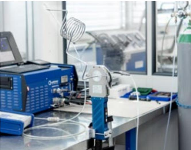
Orbital welding of tubes or of entire assemblies is also part of the range of in-house services provided by SERTO. Welding is performed automatically with a supply of inert gas with residual oxygen measurement in order to ensure the flawless quality of the welding seam.
