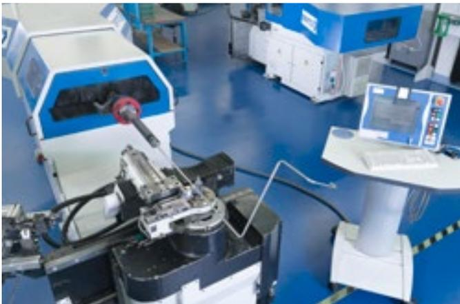
Using different bending procedures and techniques, the ultra-modern 10-axis bending centres and our many years of experience enable us to implement virtually all bending geometries, and that includes the bending of internally electropolished stainless steel tubes.
