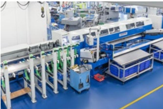
Modern, fully automatic tube saw for up to 3,000 cuts per hour with accuracy of  $\pm 0.2$  mm.
